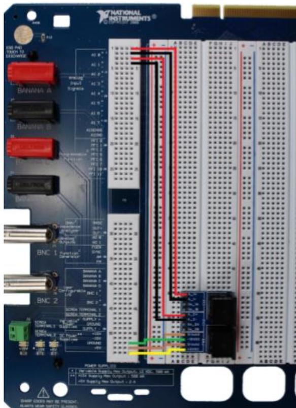
*Figure 2: NI elvis II with connections*
