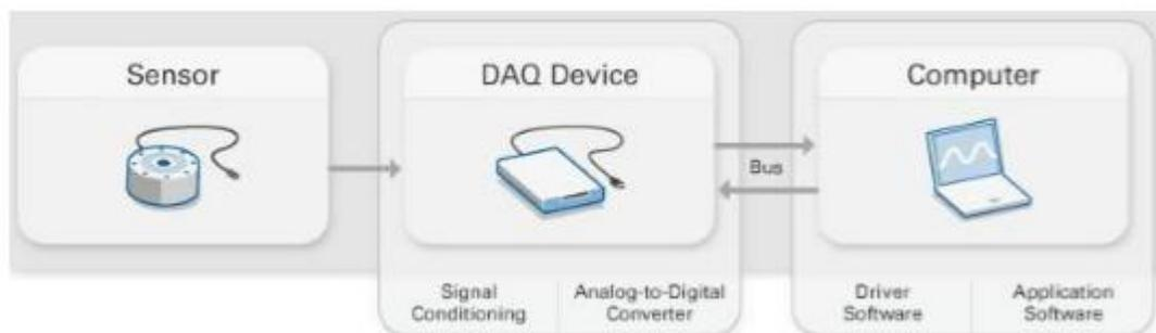
Figure :1 Data Acquisition system
