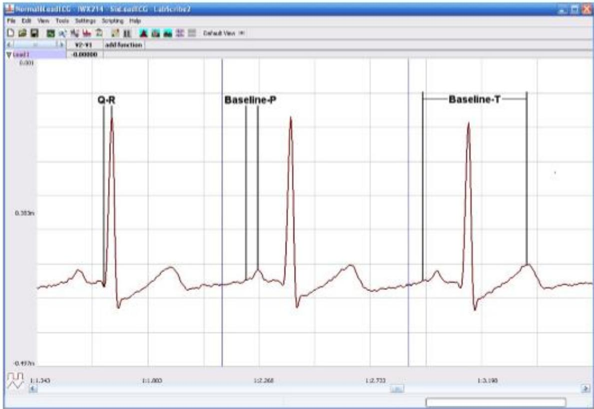
Figure 5: ECG recording displayed in the Analysis window. Lines and labels were added to indicate the locations where cursors should be placed to measure the amplitudes of R (Q-R), P (Baseline-P), and T (Baseline-T) waves.
