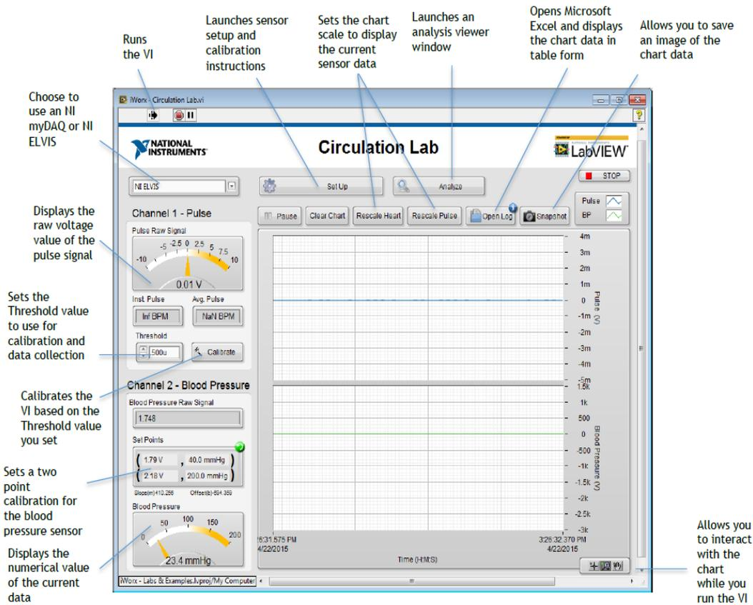
In LabVIEW, you can select <Ctrl-E> to view the block diagram, or code, of the lab VI and the annotations that explain how it works.
