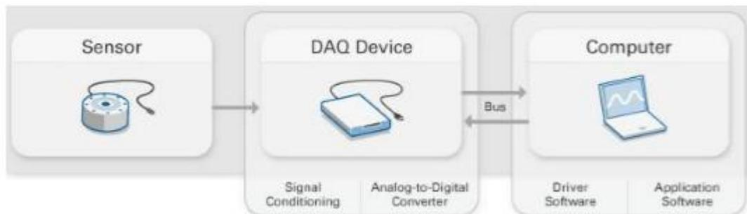
Figure :1 Data Acquisition system
