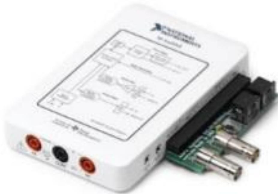
If using the myDAQ, connect the iWorx myDAQ adapter to the myDAQ device and then connect the respective sensor for each lab to Channel 1 of the adapter. When you are using two sensors, you can use Channel 1 and Channel 2 at the same time. Be sure to select the channel that you want to read in the LabVIEW software program.
