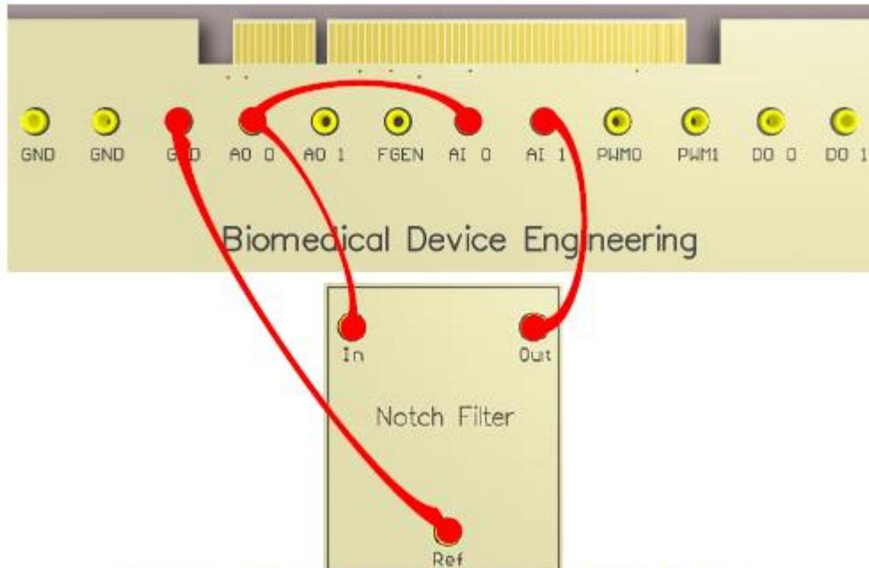
Fig. 9.3-9 Filtration circuit of generated ECG signals using Notch filter
