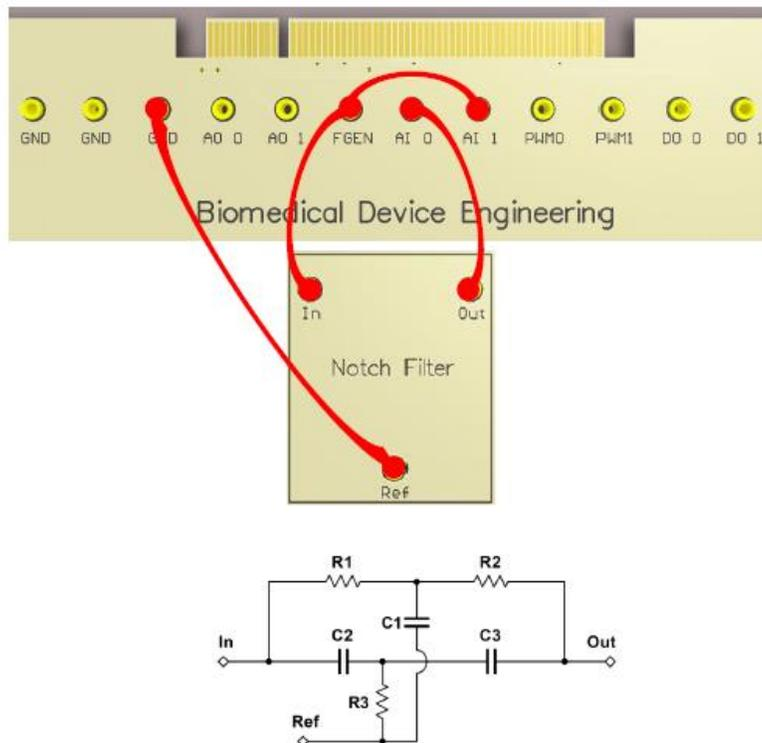
Fig. 9.3-7 Registration circuit of Bode graphs of notch filters
