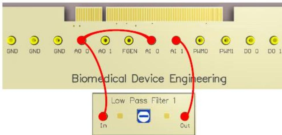
Fig. 9.5-17 Filtration of generated ECG signals using active low pass filter
