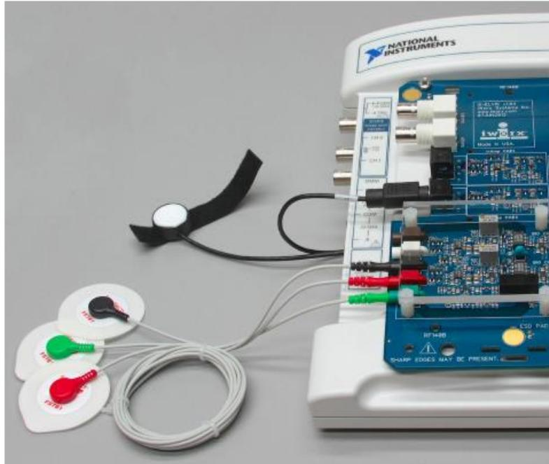
*Figure CP-1-S3: The ECG leads and pulse transducer connected to an IX-ELVIS.*
