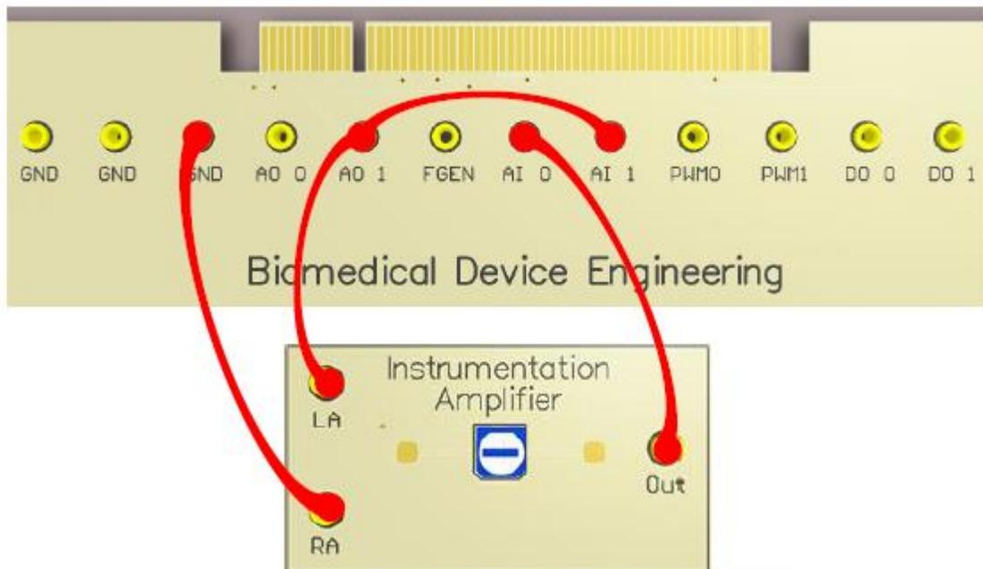
**Fig. 9.1-7 Amplification circuit of generated signals**
