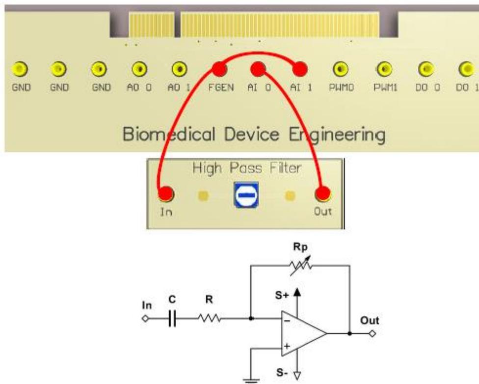
Fig. 9.5-15 Registration circuit of the Bode graphs of a high pass filter
