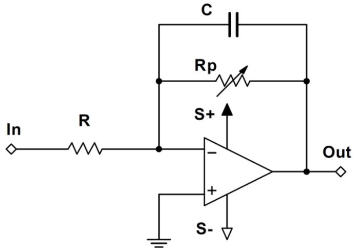
3. Turn the knob of the variable resistor **R<sub>p</sub>** of the Low Pass Filter 1 on the **Biomedical Device Engineering** board up to its mean position.
