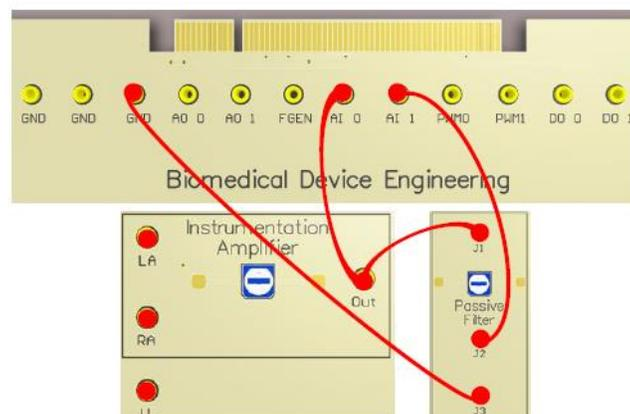
Fig. 9.4-16 Pre-amplification and filtration circuit of the ECG signals of the passive low pass filter
