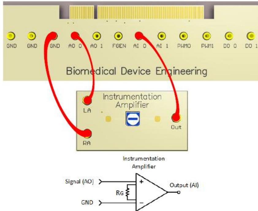
Fig. 9.2-7 Amplification circuit of generated ECG signals
