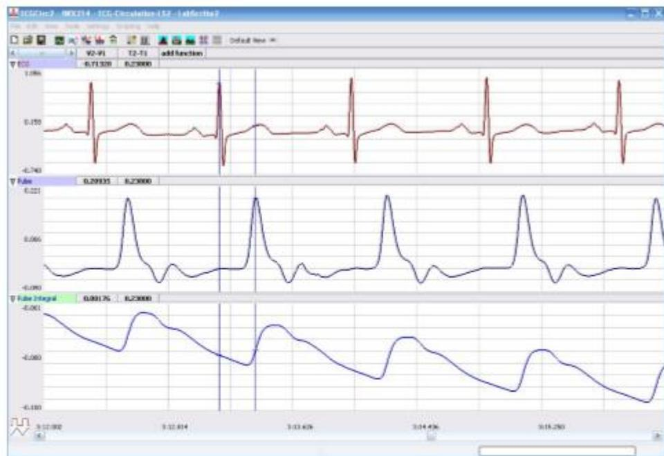
*Figure CP-1-L3: ECG, pulse and pulse integral displayed on the Analysis window with cursors in place to measure the R-Pulse interval with the T2-T1 function.*
