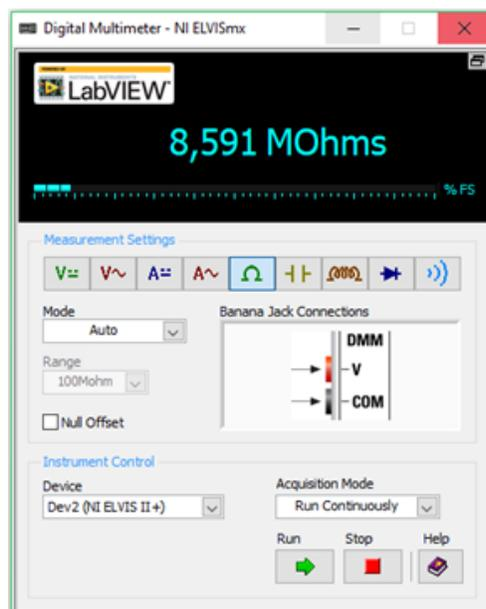
23. Using the **DMM** probes measure the resistance of the variable resistor **RG** of the instrumentation amplifier.
