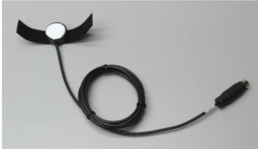
*Figure CP-1-S1: The PTN-104 pulse plethysmograph.*
