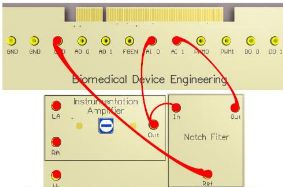
Fig. 9.3-11 Pre-amplification and filtration circuit of ECG signals using a notch filter
