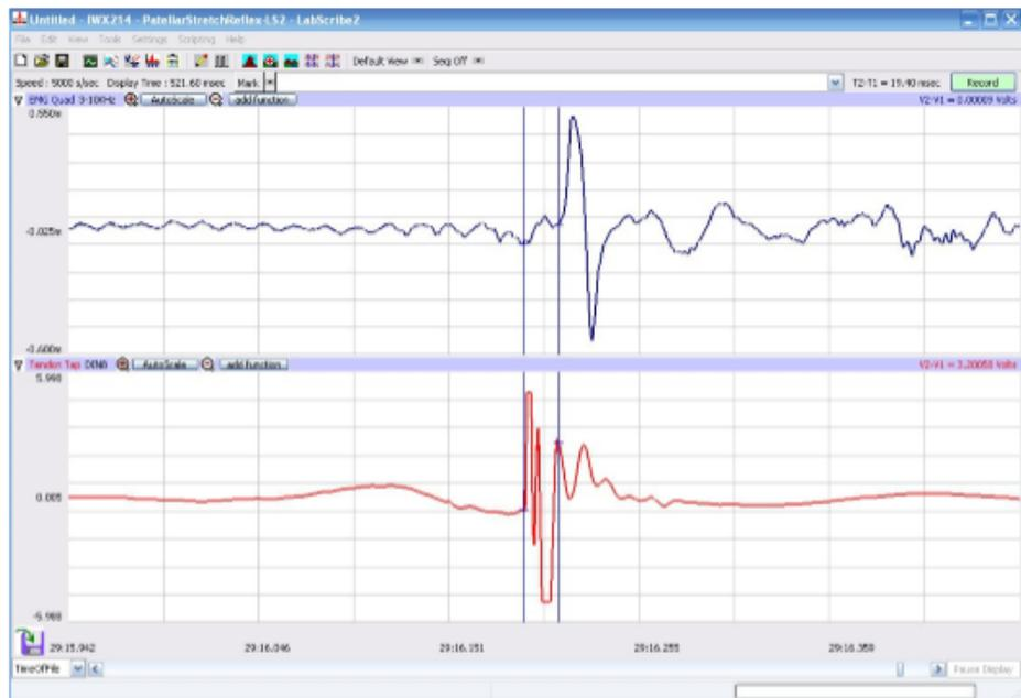
*Figure NP-2-L1: An Achilles tendon reflex response and patellar hammer signal displayed on the Main window. The cursors are in position to measure the reflex conduction time*
