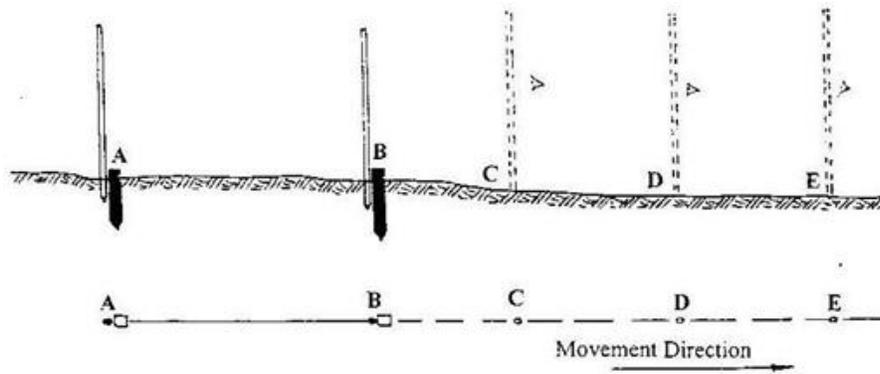
Figure 1.1. Setting out points on the extension of two fixed points.
