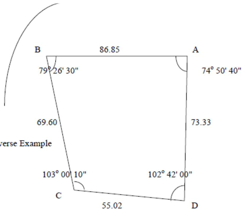
Fig. 9.1 Closed Traverse Example
