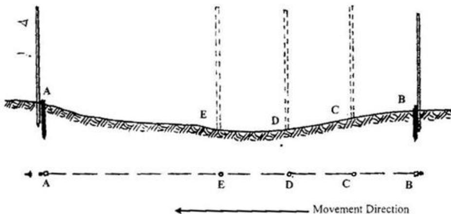
Figure 1.2. Setting out points between two fixed points.
