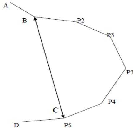
Figure 10.2b Closed traverse between two fixed points
