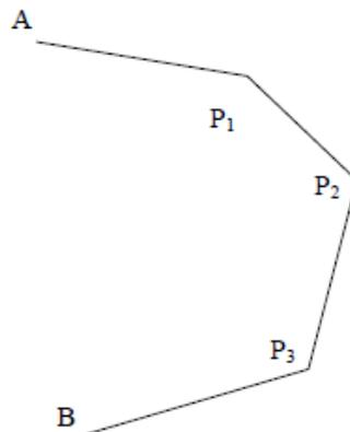
Figure 10.1 Layout of an open traverse
