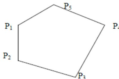
Figure 10.2a Closed Loop traverse
