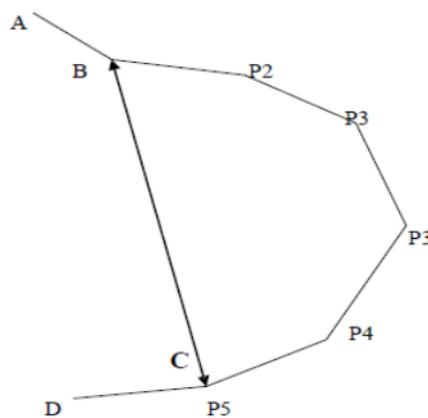
Figure 11.1b Closed traverse between two fixed points
