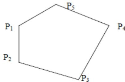
Fig 11.1a Closed Loop traverse
