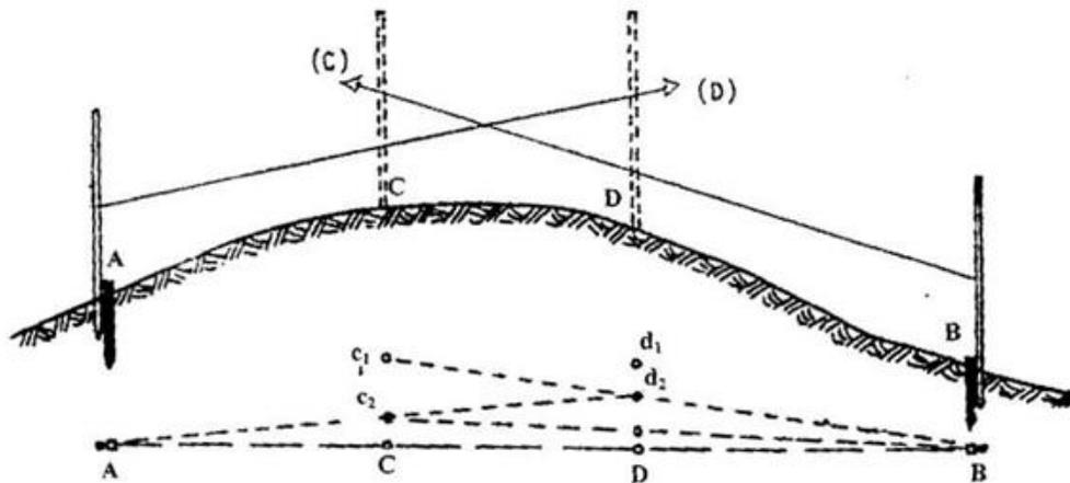
Figure 1.3. Setting out points between two points separated by high ground.
