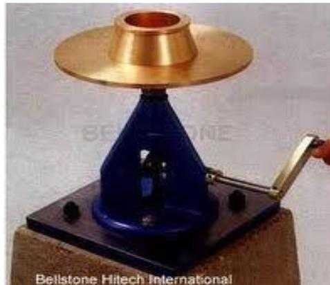
g) Use calipers to measure the diameters along the 4 scribed lines on the table. The sum of the four readings is the flow (the percent increase in the original diameter). Record this flow value.
