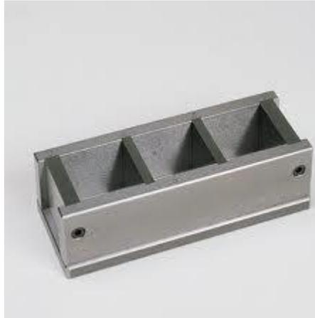
1) Place a layer of mortar about 1 in. (25 mm) (approximately one half of the depth of the mold) in all of the cube compartments.
